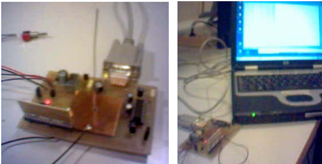
Figure 73. Left: Final form of the receiver circuit of the wireless DAQ system, right: receiver circuit hooked to a PC
