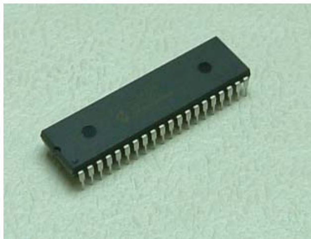
Figure 13. The look of a microcontroller - just like any other IC – here Microchip PIC 16F74 (Ref.[37])
