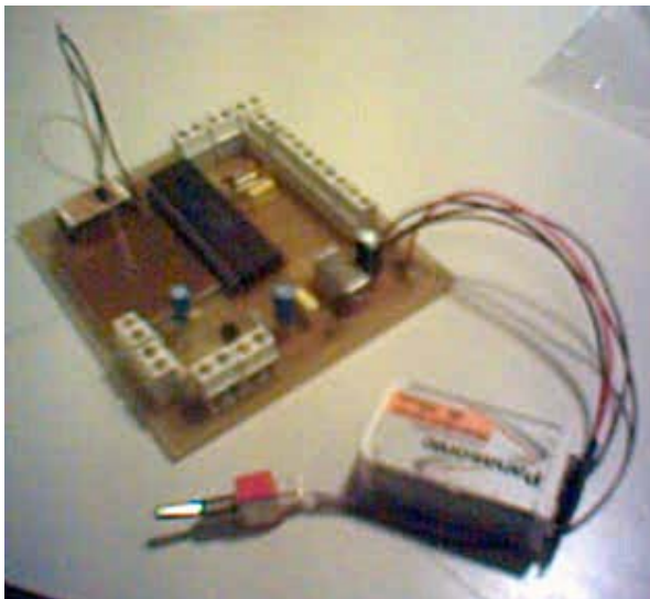
Figure 70. Final form of the transmitter circuit of the wireless DAQ system
