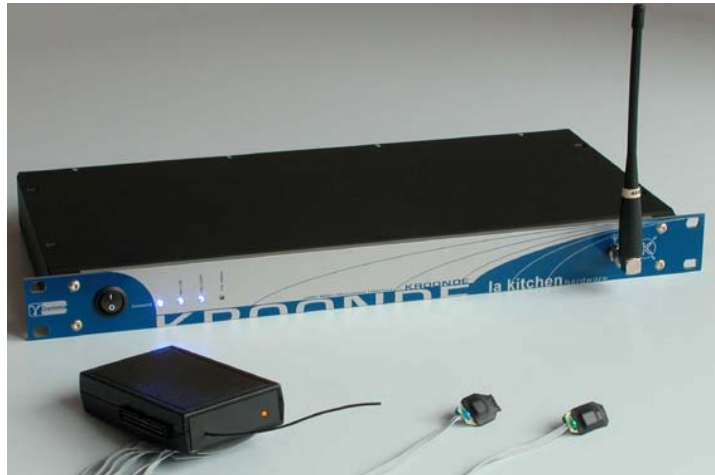
Figure 2. The Kroonde Gamma - a receiver (blue 1U rack), portable transmitter (black box), and sensors (Ref. [18])
