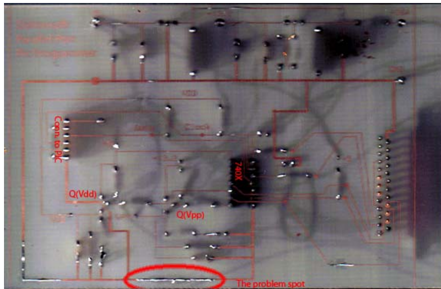
Figure 31. The back side of the hardware programmer developed in this project, indicating a broken track problem
